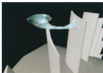
Fig. 11 Illustrations for flow structure of short length-scale stall cell
